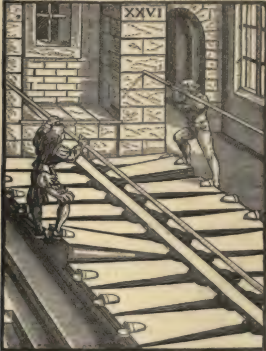
BELLOWS OF THE HALBERSTADT ORGAN, 1301, SHOWING THE IRON SHOES BY WHICH THE BLOWERS RAISED THE UPPER PLATES.
